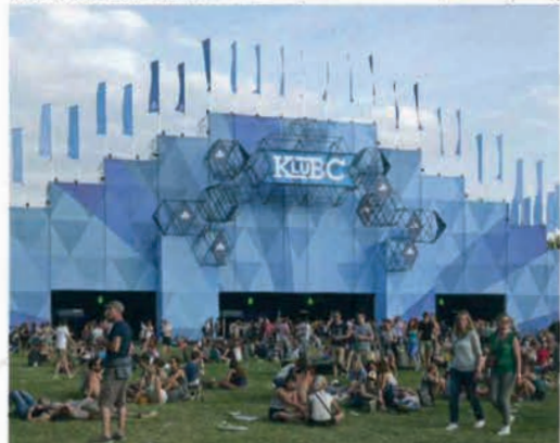
KBC Festival - Belgium: Sublimation imprint method, THD 5 m width on 240g fabric. Three times lighter than canvas, easy to install and store, and more environmentally friendly.
